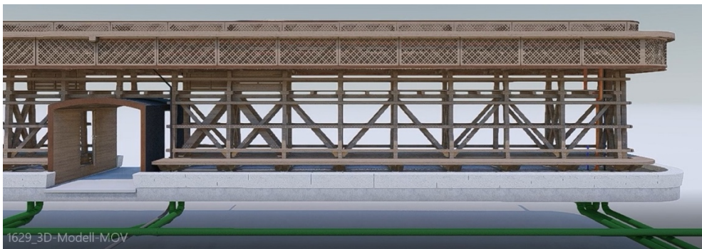
Fig. 3: Coordination basic pipework, concrete construction, wooden construction
