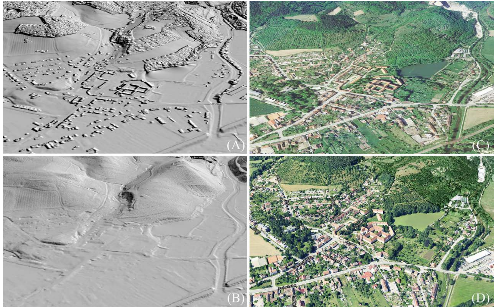
Fig. 3: (A) Digital surface model DMP 1G – LOD 3 maps, (B) digital terrain model DMR 5G – LOD 2 maps, (C) Google Maps 3D view, (D) Mapy.cz 3D view
